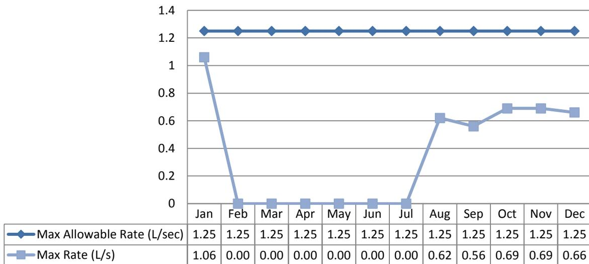
Note: Well 4 not in production other than for sampling: January, March, April, May, June, July, September and November. The spike in January was due to scheduled Flow Meter calibration.
