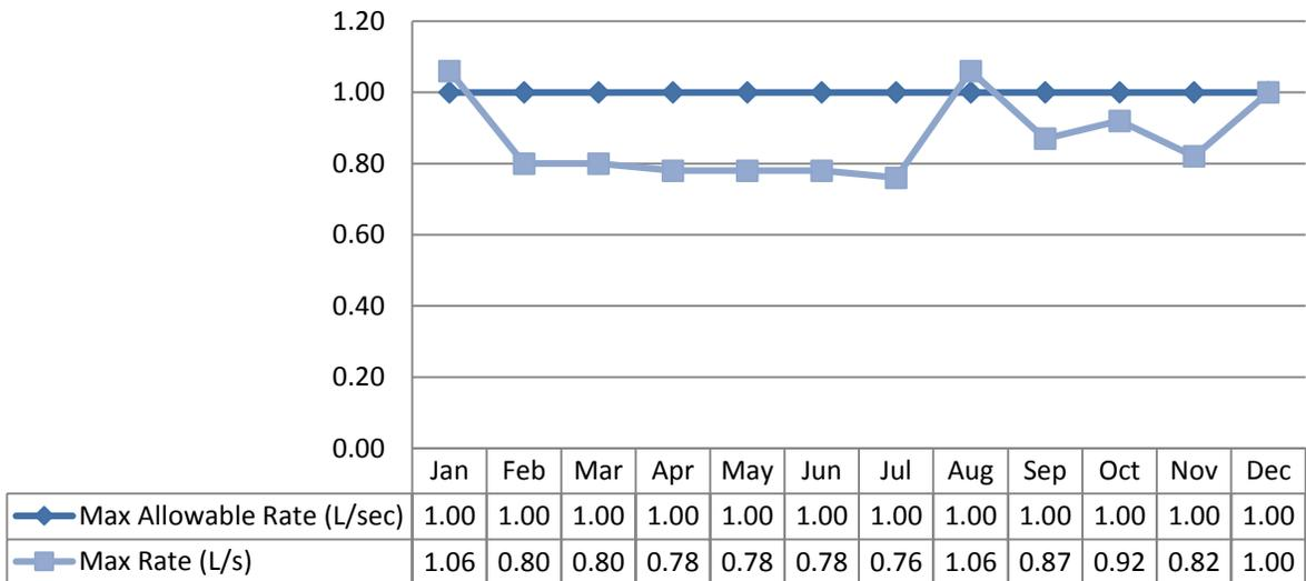
Note: The above table shows there were exceedances in instantaneous peak flow rate (L/s) this is due to well pump start-up. The spike in January was due to scheduled Flow Meter calibration. The spike in August was due to troubleshooting/maintenance. All spikes are reviewed for compliance.
