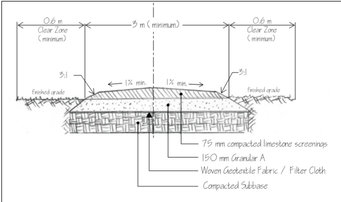
**Figure 4.10: Limestone Screenings Surface Cross-Section, General Application**
