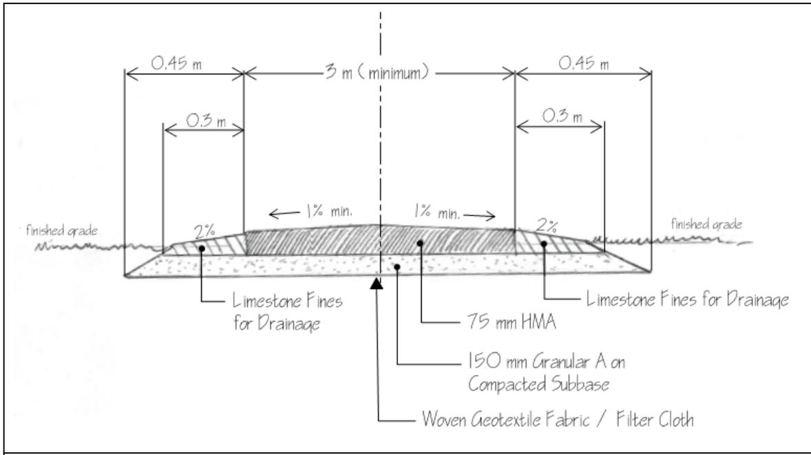
**Figure 4.9: Asphalt Trails, Separate from Road**
