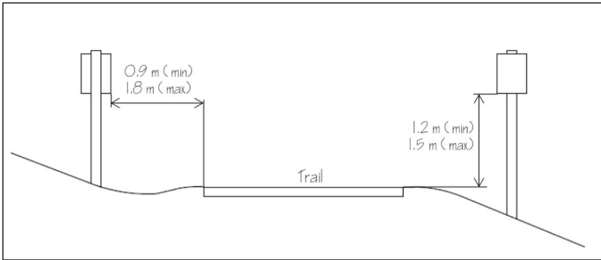
**Figure 4.12: Sign Installation**
