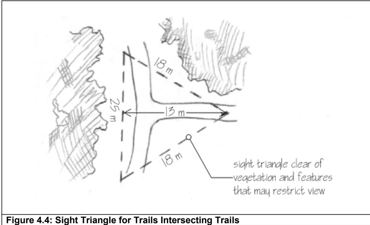
**Figure 4.4: Sight Triangle for Trails Intersecting Trails**
