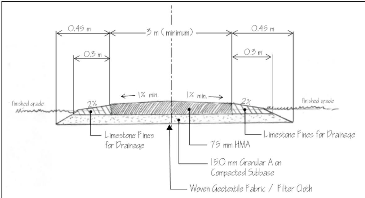
**Figure 4.9: Asphalt Trails, Separate from Road**
