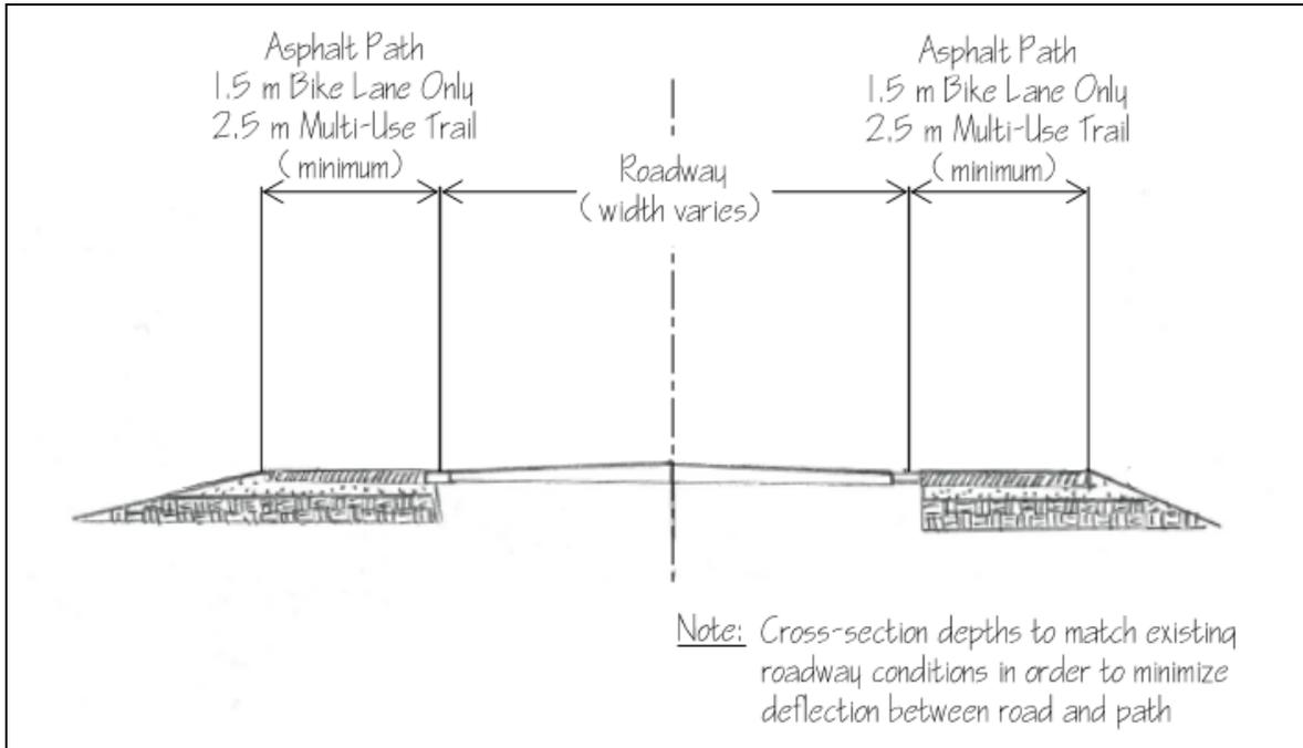
**Figure 4.8: Extended Asphalt Shoulder Trails (Bike Lanes)**
