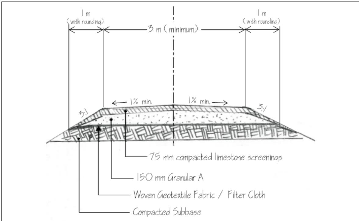
**Figure 4.11: Limestone Screenings Surface Cross-Section, Abandoned Rail Lines Application**
