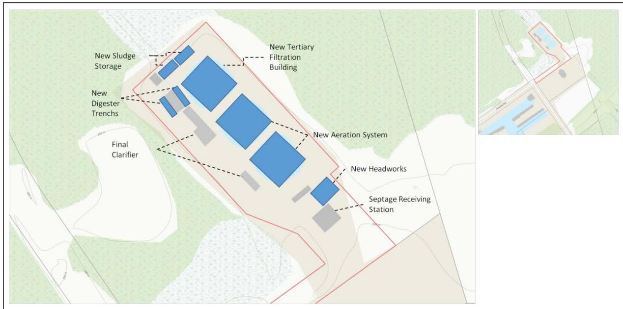
*Figure 4: Site Overview with upgrades to expand plant capacity identified*
